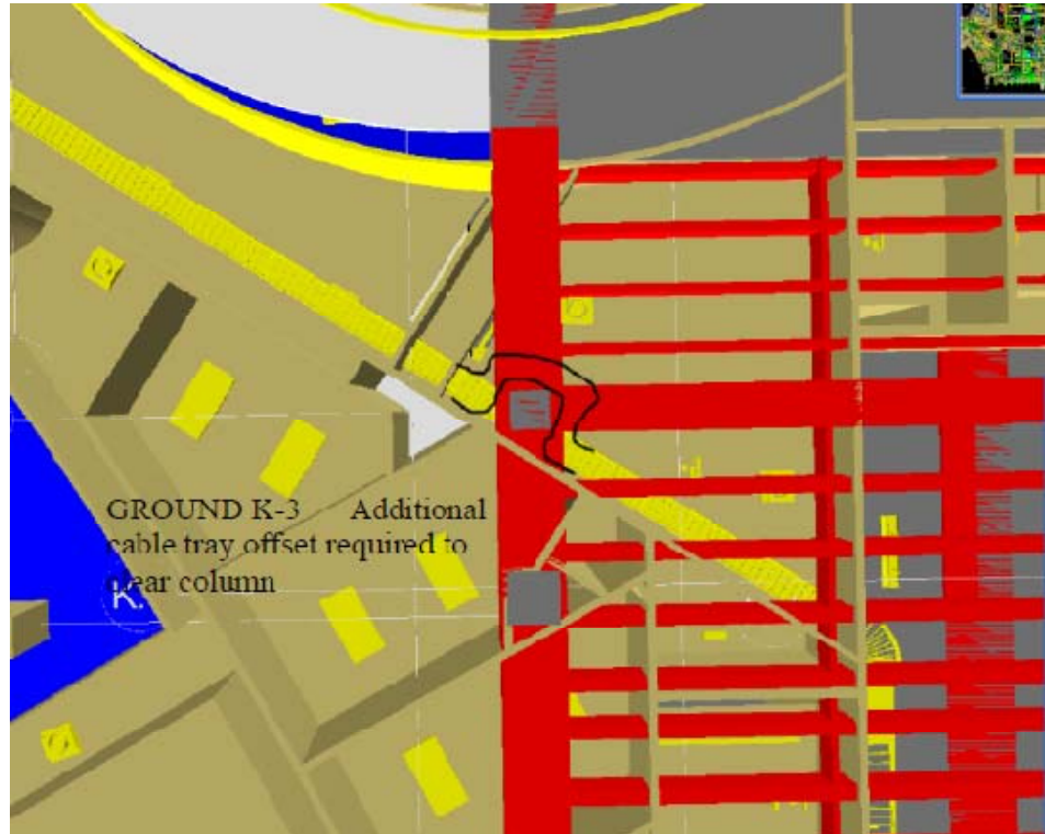
Figure 7.23: Example 10 – Reroute Cable Tray to Clear Column
